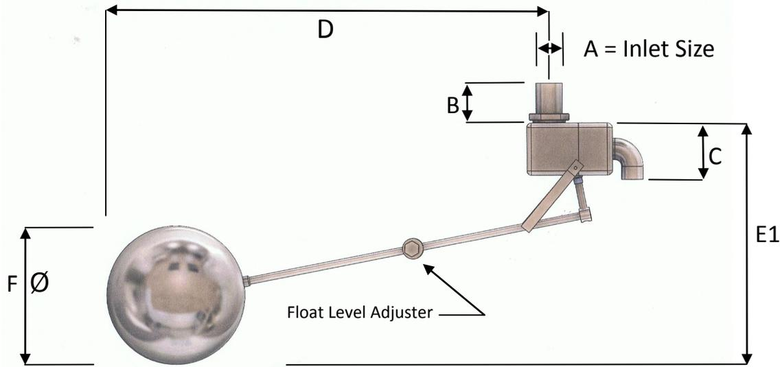
E1 Denotes Closed Position      Valve is shown in Closed Position
